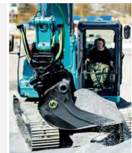
3 auxiliary lines as standard make working with tiltrotators easy
