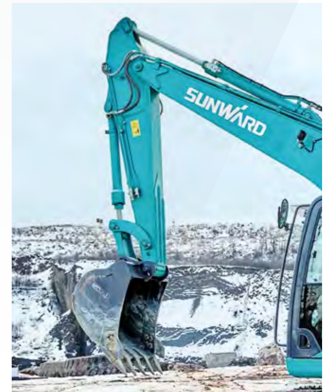
The swing arm and bucket rod are designed with the reliability standard of 20 000 hours.
